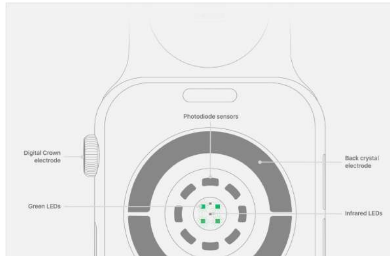
Figure 18. heart rate detection method with PPG sensor
