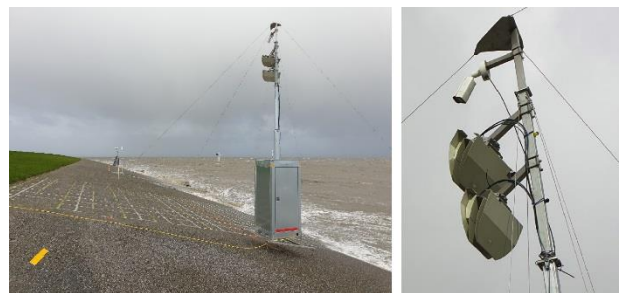
Figure 2 - Left: New laser scanner system next to the overtopping tanks on the dike in the Eems-Dollard estuary. Right: from the bottom to the top: Laser scanner 1, laser scanner 2, video camera.
