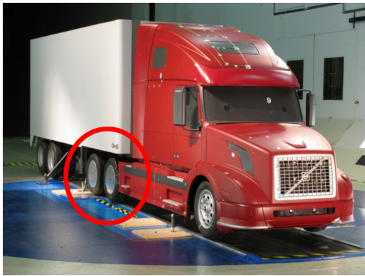
Figure 2.39: Model with hub caps fitted
