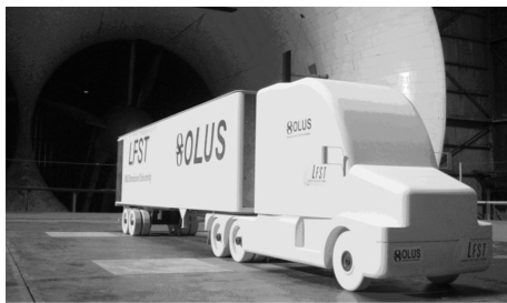
Figure 2.25: Side-skirts with covered and uncovered wheels (Credit: Van Raemdonck 2012 )
