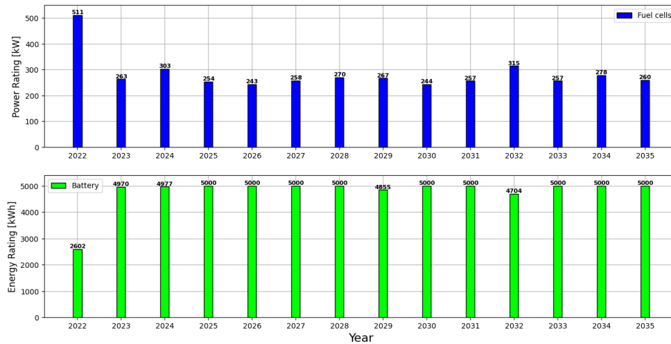
Figure 6.19: Optimal power/energy ratings based on the lowest TCO for the second scenario
