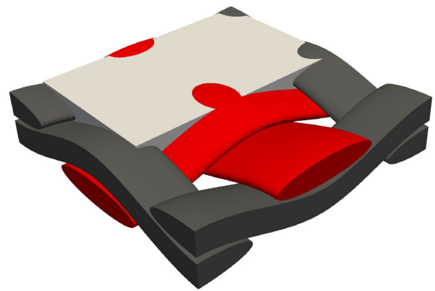
Fig. 1 Fiber composite weave with two types of fibers and a binding matrix material. The matrix material is shown in off-white and partially removed for better visibility
