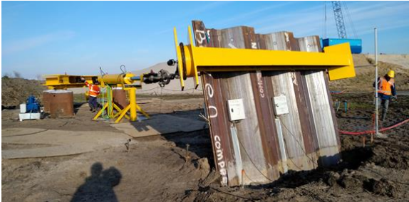
Figure 4. Photo of AZ13-700 during the test
