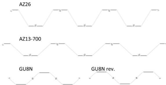
Figure 2. Sheet pile profiles
