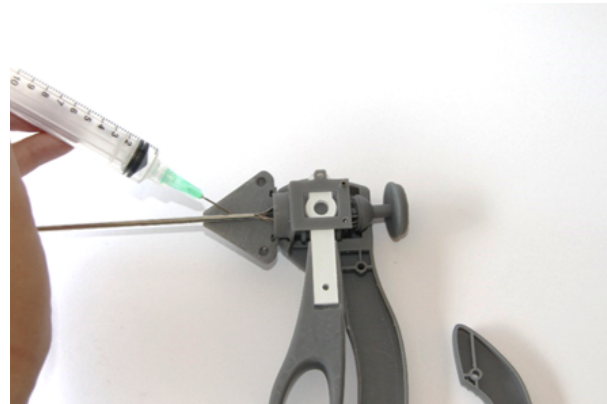
25. Place first half of the roticulator and apply glue
