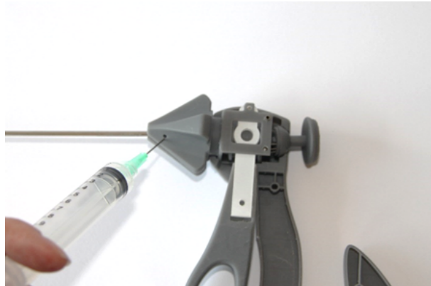
26. Place other half of the roticulator and apply more glue through the glue hole
