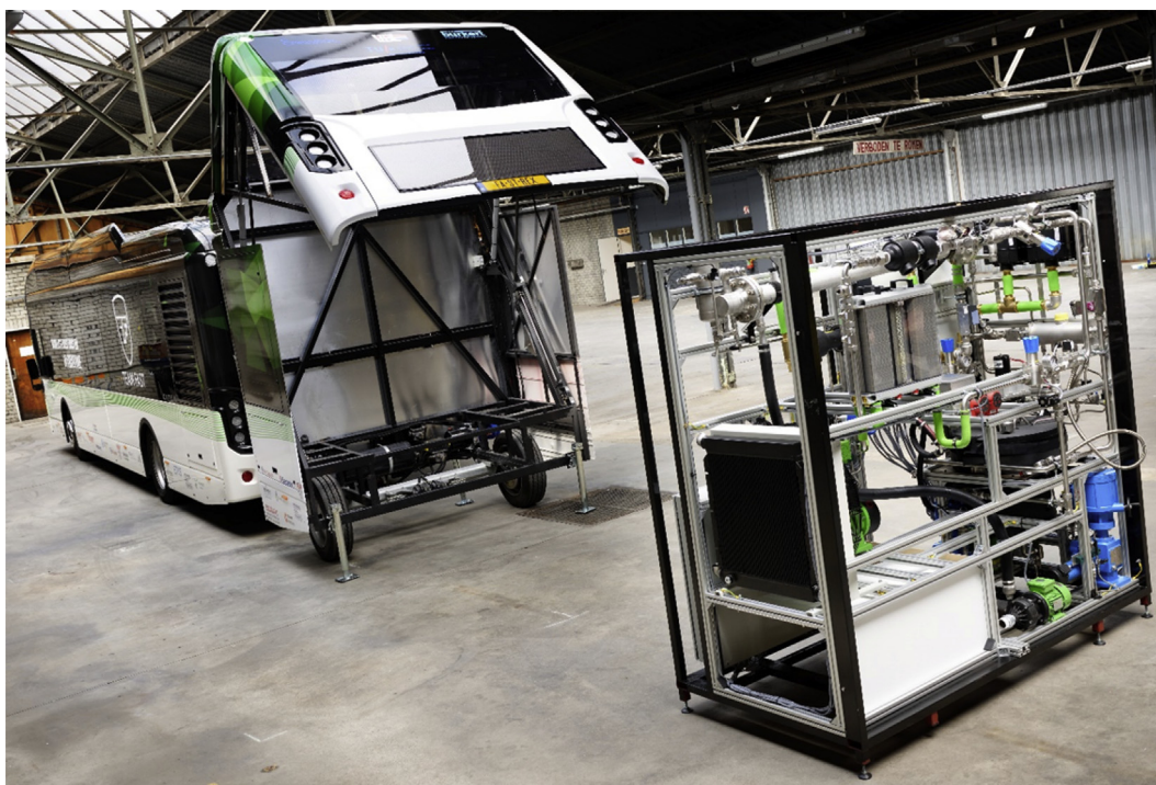
Fig. 4 – Implementation of 25 kW system in full-scale hydrogen powered city bus.
