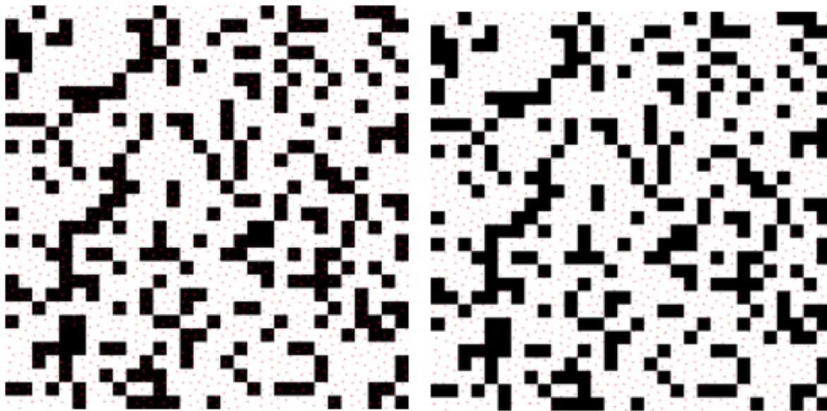
Figure 3.20: The points received from the point generation components, do not match with the high-resolution vegetation map. Therefore, it is necessary to throw away the points that are in the black pixels of the detailed vegetation map. The left image overlays the point distribution with the high-resolution vegetation map and on the right all points that were in the black pixels are removed.
