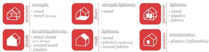
Figure 9. Lightweight materials characteristics and applications
