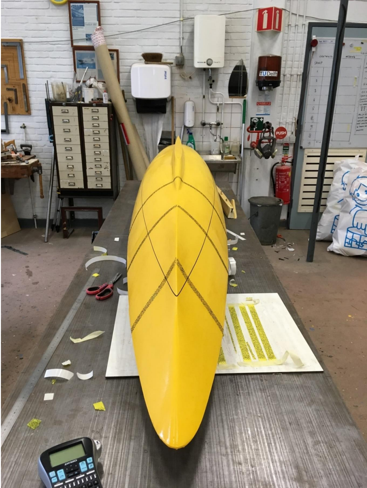
New turbulence strips were made and applied on the hull of the model.
