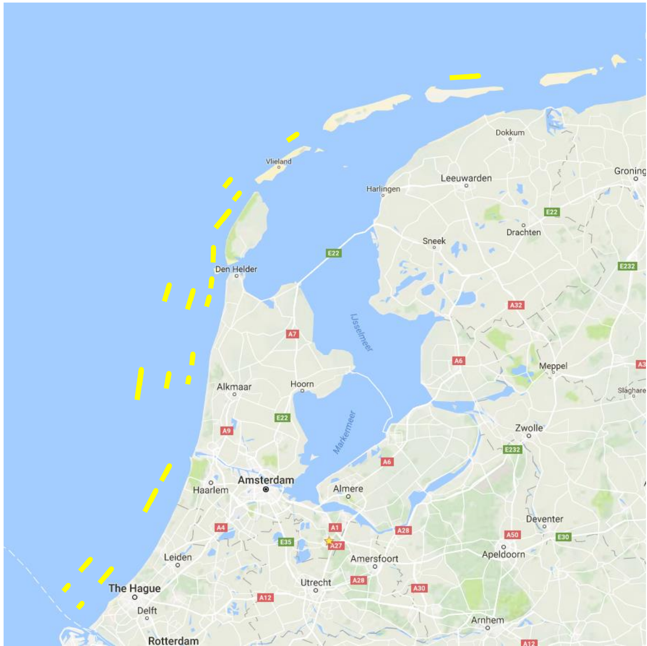
Figure 21: Overview of selected shoreface nourishments. When two or more shoreface nourishments are executed at the same location, the first one executed in time is the one closest to the coast. The second one is represented by the next one in row and so on. I.e. the shoreface nourishments are alongshore on the exact location, but cross-shore they are based on their execution phase and not the cross-shore distance to the coast. (Source of map: google.com)
