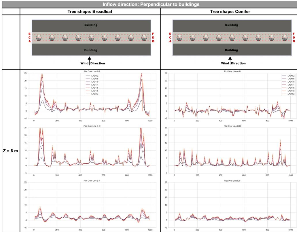
Figure 5.13.:  $C_{12-13}$  values on three probe lines at 6 m height within the street canyon (perpendicular inflow direction)
