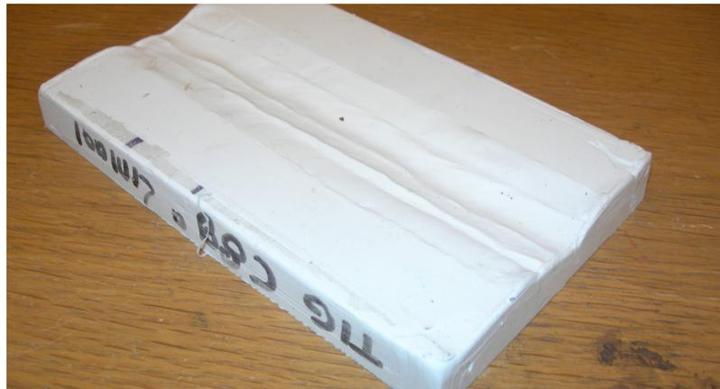
figure 5.4 Silicon rubber cast of C89a plate
