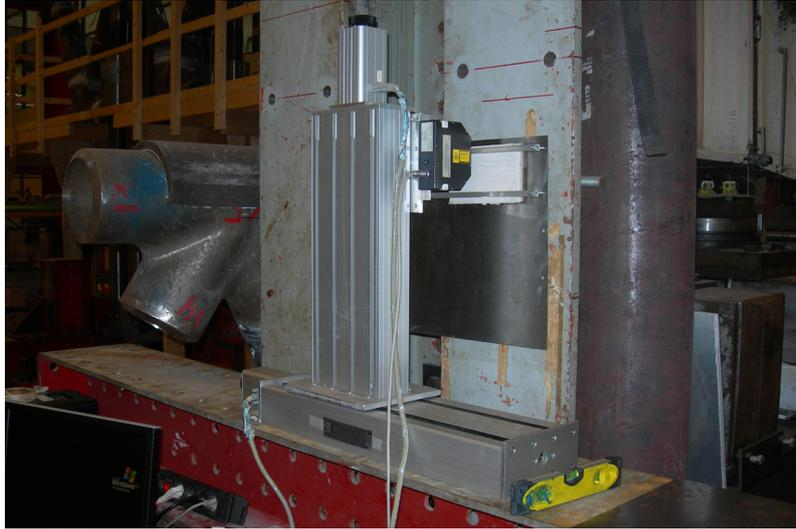
figure 5.1 Setup to measure the geometry of welds
