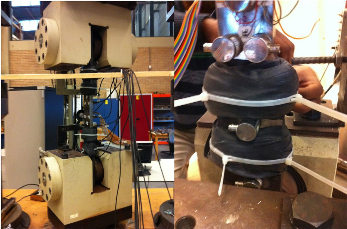
**figure G.1 Left: test setup with sensors and dampers applied to the specimen. Right: close up of three sensors without any cables attached and two dampers made of plasticine, pretensioned with bicycle tires.**
