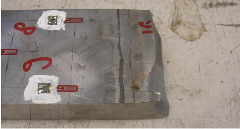
figure 9.2 Backside of specimen C69-1 with sharp notches at the weld root
