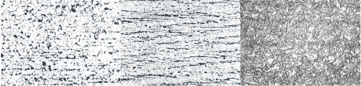
figure 2.3 From left to right; microstructures of normalized S460, thermomechanically rolled S460 and quenched and tempered S1100 (source: VM publication 125, 2008)
