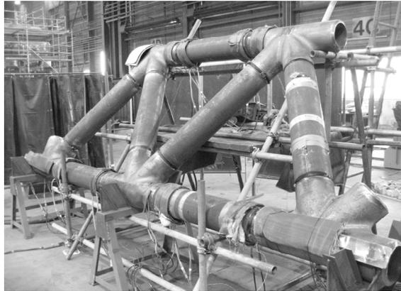
figure 2.13 A truss with cast steel nodes (source: Pijpers et al., 2010)
