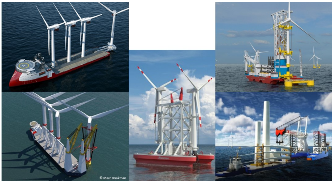
Figure B.11: Selection of new concepts, showing Windlifter (top left) [156], WTS (middle) [157], WIV (top right) [158], PWT (bottom left) [48] and Feederdock (bottom right) [159].
