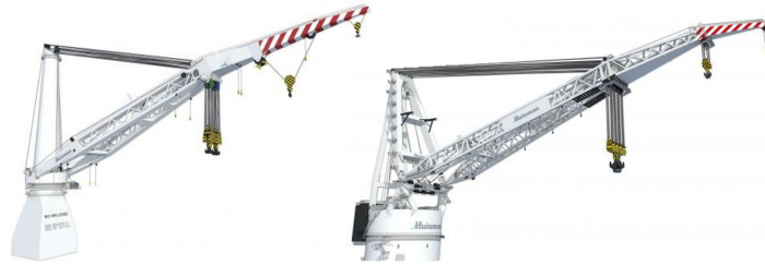
Figure 3.4: Artist impressions of mast crane (left) and tub mounted crane (right), from Huisman .
