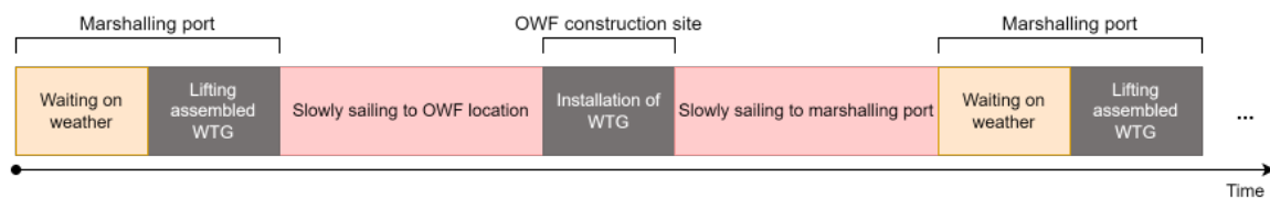
Figure B.7: Timeline showing the T&I process for a sheerleg. The timeline is not to scale. The bottleneck is shown in red.
