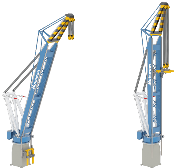
Figure 3.5: An impression of the Zephyr crane concept, received from Huisman . The left render shows the free-hanging mode, while the right shows the guided lift mode.
