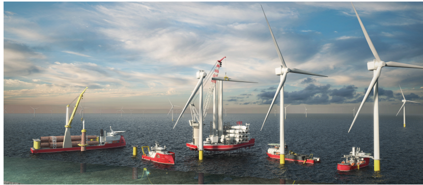
Figure 1.6: General overview of the ships involved in the installation of an OWF with monopile foundations.
