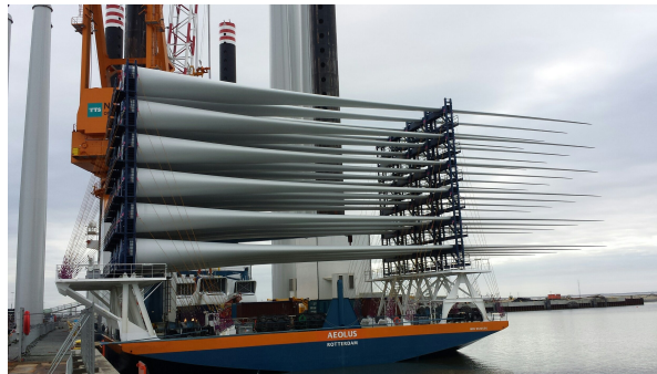
Figure 3.9: Picture of the blade rack on Aeolus , from [79].
