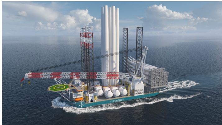
Figure 6.1: Render of an NG-20000X jack-up, currently under construction for Havfram . From [104].
