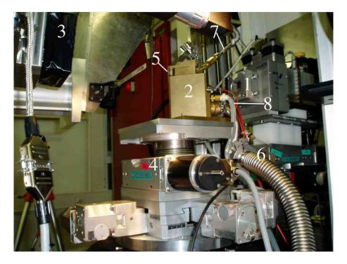
**Figure 6.2:** Experimental set-up used for in-situ synchrotron diffraction studies at the ID-11 of ESRF. 1. beam entry slit, 2. 3D-XRD furnace, 3. 2D FreLon<sup>TM</sup> area detector, 4. x-y-z- $\omega$  table, 5. sample chamber, 6. vacuum circuit 7. helium inlet via mass flow controller, 8. water cooling circuit.
