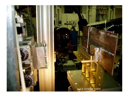
Figure 5.5: Synchrotron X-ray diffraction set-up used for welded TRIP steel plates. The white line indicates the measurement line.
