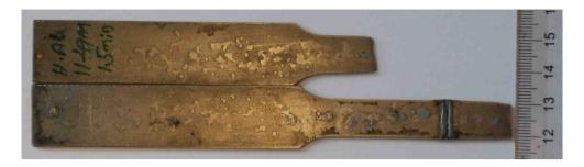
Figure 7.4: A welded High-Al TRIP sample tensile tested 90 s after welding showing a ductile failure in the base metal region, about 18 mm from weld centre line.
