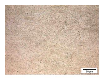
Figure 4.12: The fusion zone of a GTA welded DP600 steel does not show the presence of coarse or large amounts of inclusions, unlike the GTA welded TRIP steels. In contrast, only a few small (<1μm) inclusions were observed (little black dots in the microstructure).</p>
