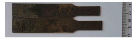
Figure 7.6: A welded High-Al TRIP sample tensile tested 900 s after welding showing a complete brittle failure at the centre of the weld.
