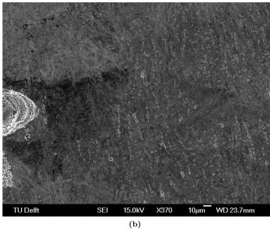
**Figure 4.14:** Secondary electron image showing the inclusion density at the prior weld plate interface. The cavity indicates the plate interface at the overlap position and the white lines show the inclusion distribution (a) and (b) with higher magnification.
