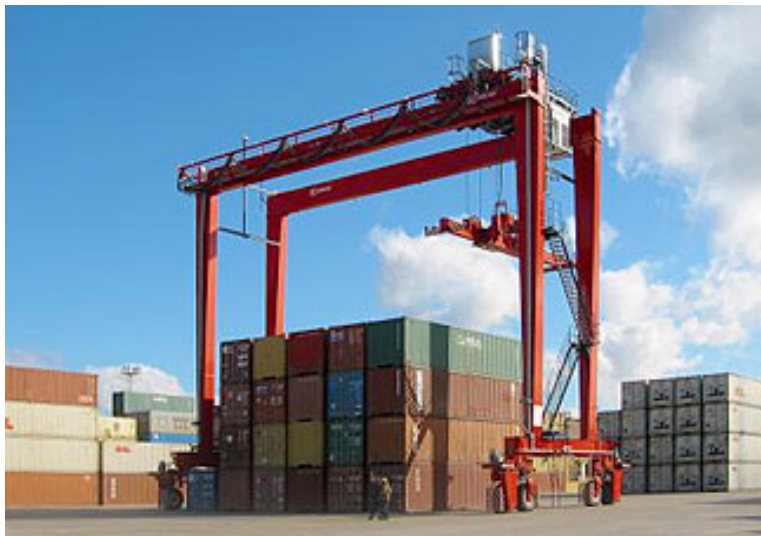
Figure 7.31: Rubber Tyred Gantry (RTG) (source: Kalmar)
