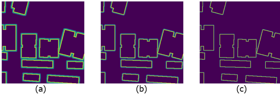
Figure 5.4: Border weight maps when using fixed w_0 = 10 and different \sigma_0 values: (a) \sigma_0 = 0.2 , (b) \sigma_0 = 0.5 , (c) \sigma_0 = 0.8
