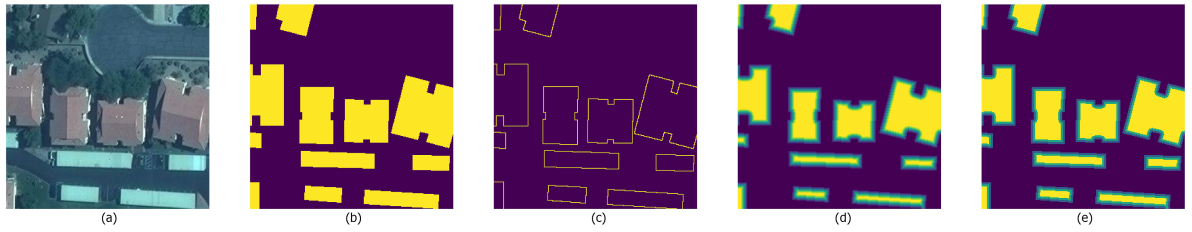
Figure 6.1: Steps to obtain the multi-level boundary label. (a) Satellite image, (b) Binary label, (c) Building boundaries, (d) Truncated distance map, (e) Multi-level boundary label.
