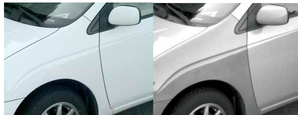
Figure 1.2: a white Toyota Prius with a new replaced fender imaged by visible light (left) and UV light (right).
