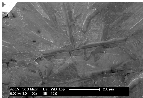
(c) A junction where two etched-out cracks meet. Cracks and flaking are visible on the surrounding surface
