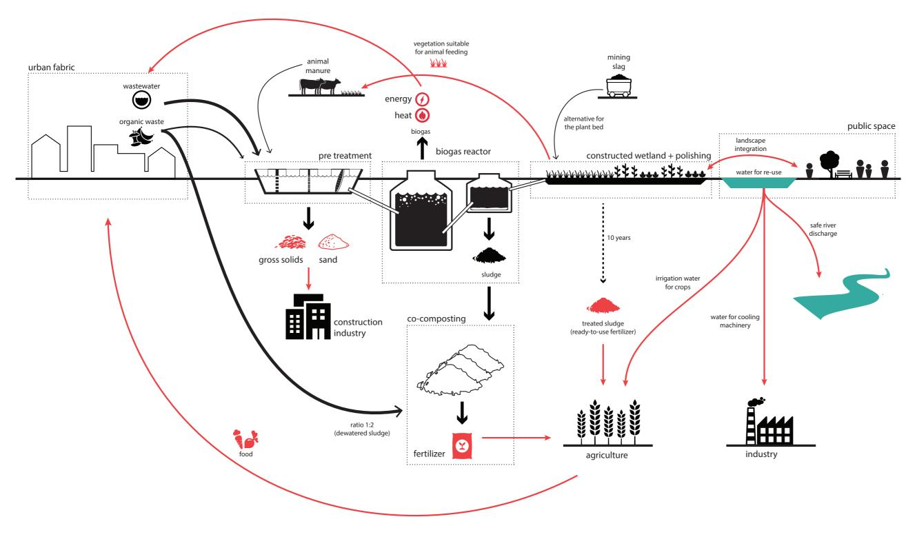
With the association of the constructed wetland with a biogas reactor and a co-composting unit, it is possible to treat wastewater and solid waste. The combination results in rich byproducts that allow interconnections between flows.
