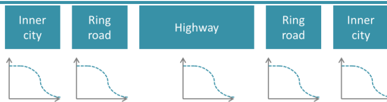
figure 3: an example of different speed flow curves to calculate the travel time between large cities in the Randstad.
