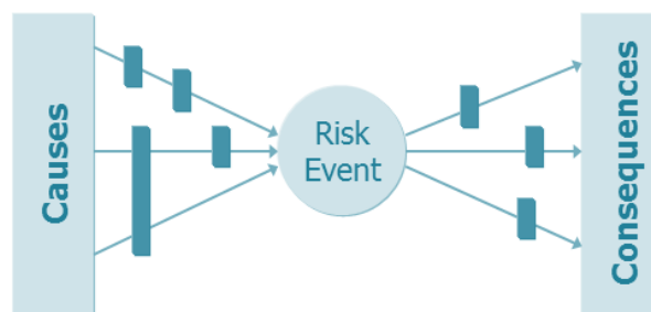
Figure 3. Risk Description and Response using a Bow Tie Method, adapted from Hillson (2014) (Hillson)
