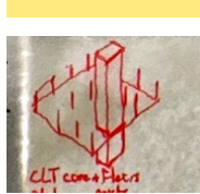
laminated core+floors + glulam post/beam
