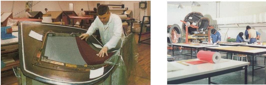
Figure 6.21: Hand lay up of prepreg composite sheets [46].
