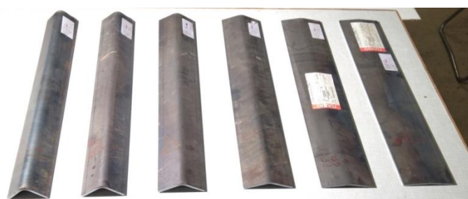
Fig. 2 4 mm thick specimens with different cold-formed angles
