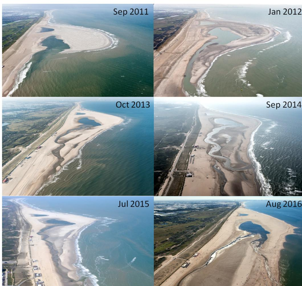
**Figure 1.** Aerial photographs of the Sand Engine in the period 2011–2016, looking south. Photographs courtesy of Rijkswaterstaat/Joop van Houdt and Jurriaan Brobbel, available through: [www.flickr.com/photos/zandmotor](http://www.flickr.com/photos/zandmotor).
