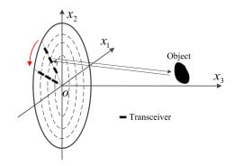
Fig. 1. Geometrical configuration of 3-D imaging with a rotating antenna array. With the rotation of the linear array, the antenna polarizations constantly change.
