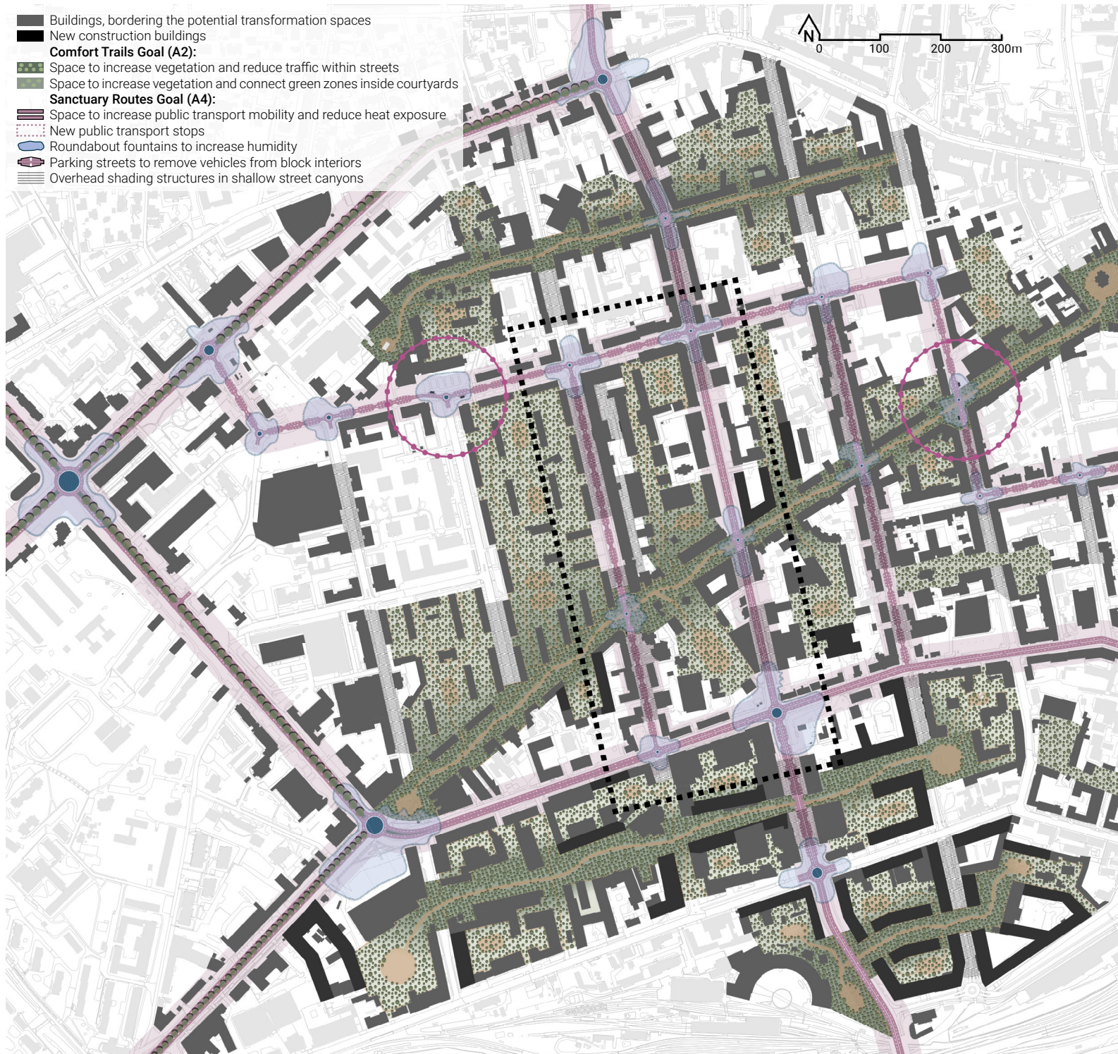
Transformation Vision for a Compact Mid-rise Environment Naujamiestis neighbourhood with possible large-scale adaptations strategies
