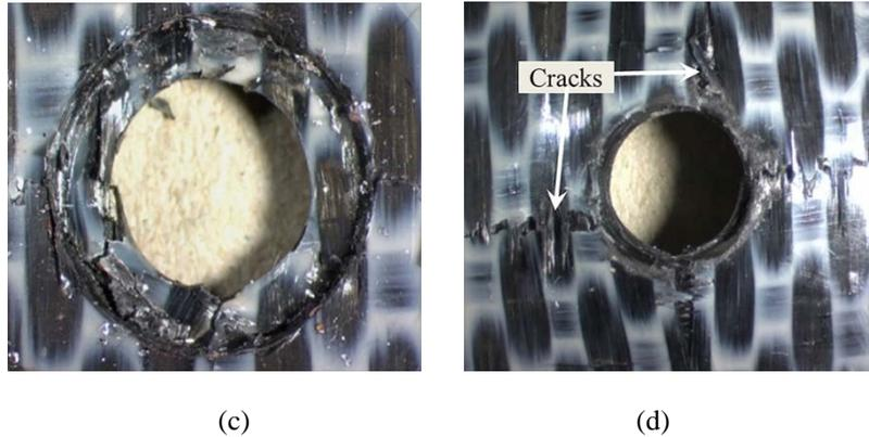
Fig. 16. The Hi-Lok<sup>®</sup> collar (HL12V6) after the PT test (a) and the side (b), bottom (c) and top (d) view of fracture surface of bottom adherend after removing the fastener.
