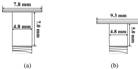
Fig. 6. Schematic of the Hi-Lok<sup>®</sup> fasteners utilized in the mechanical tests: (a) HL10V6; (b) HL12V6.
