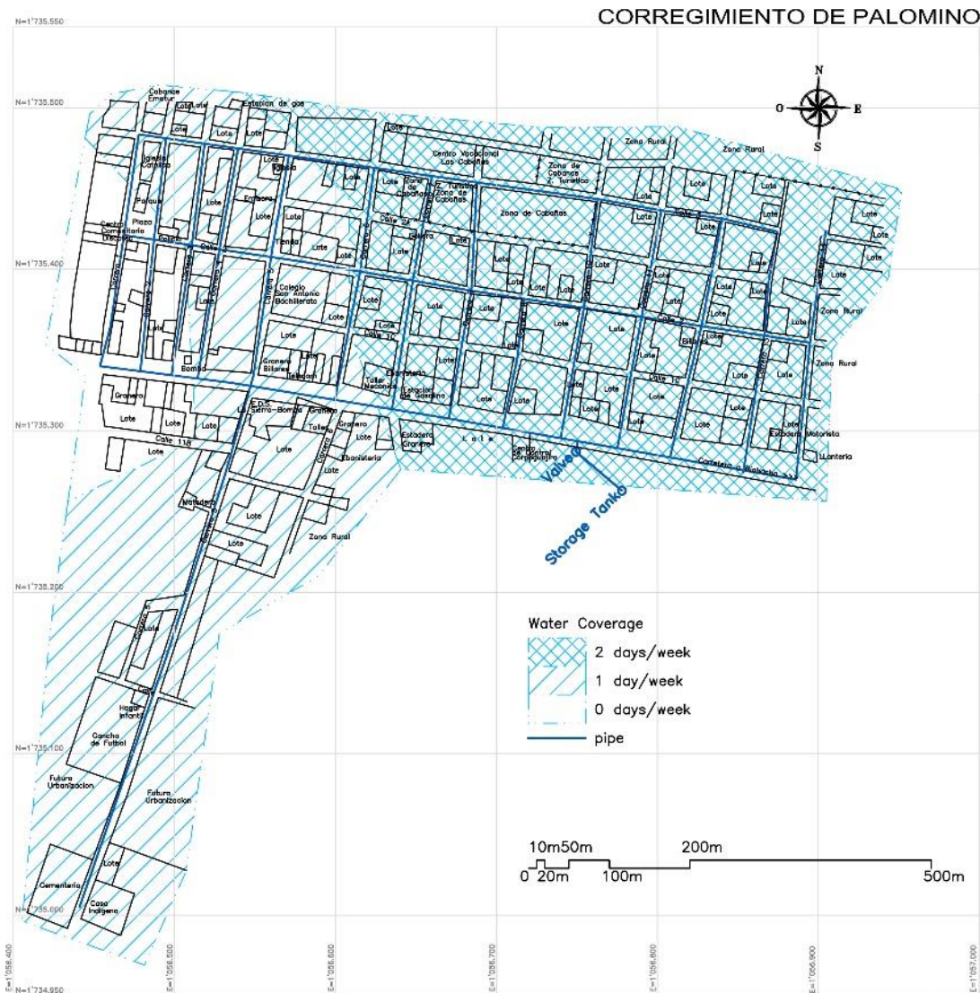
Figure 64: Main infrastructure for the centralized water system (aqueduct) and water supply coverage in days per week.
