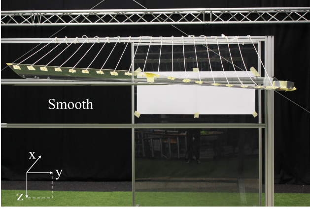
Figure 22: Ceiling set-up used for the inclined and smooth ceiling flight experiments.
