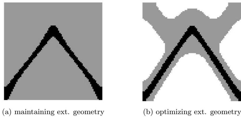
Figure 3.33: Case study n.7 - solution derived by the code developed in this thesis for reinforced concrete - no concrete cover
