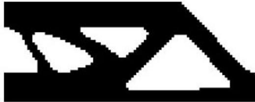
Figure 3.7: Case study n.1 - solution by Xie [11] with ESO stiffness optimization
