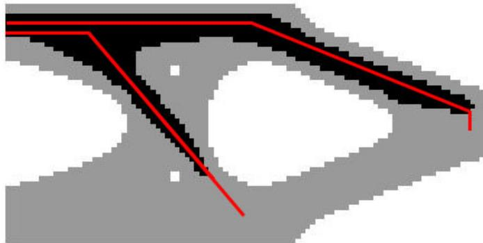
Figure 4.41: Case study n.2 - example interpretation of solution - optimized structure boundaries
