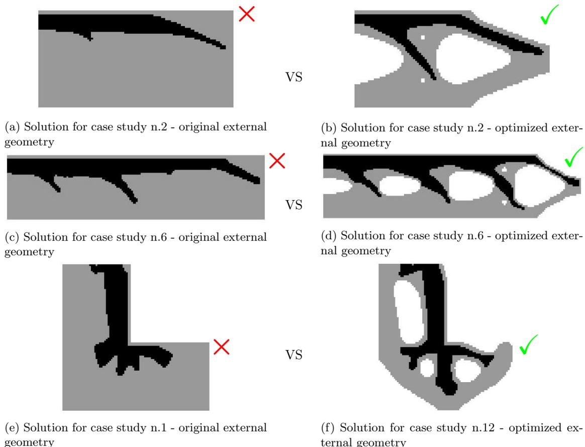
Figure 4.7: Comparison of solutions for case studies with and without “anchoring” effect of steel to holes
