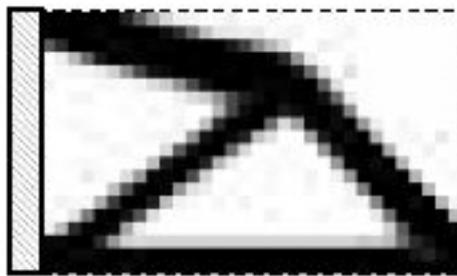
Figure 3.20: Case study n.4 - solution by Sigmund [7] with SIMP stiffness optimization
