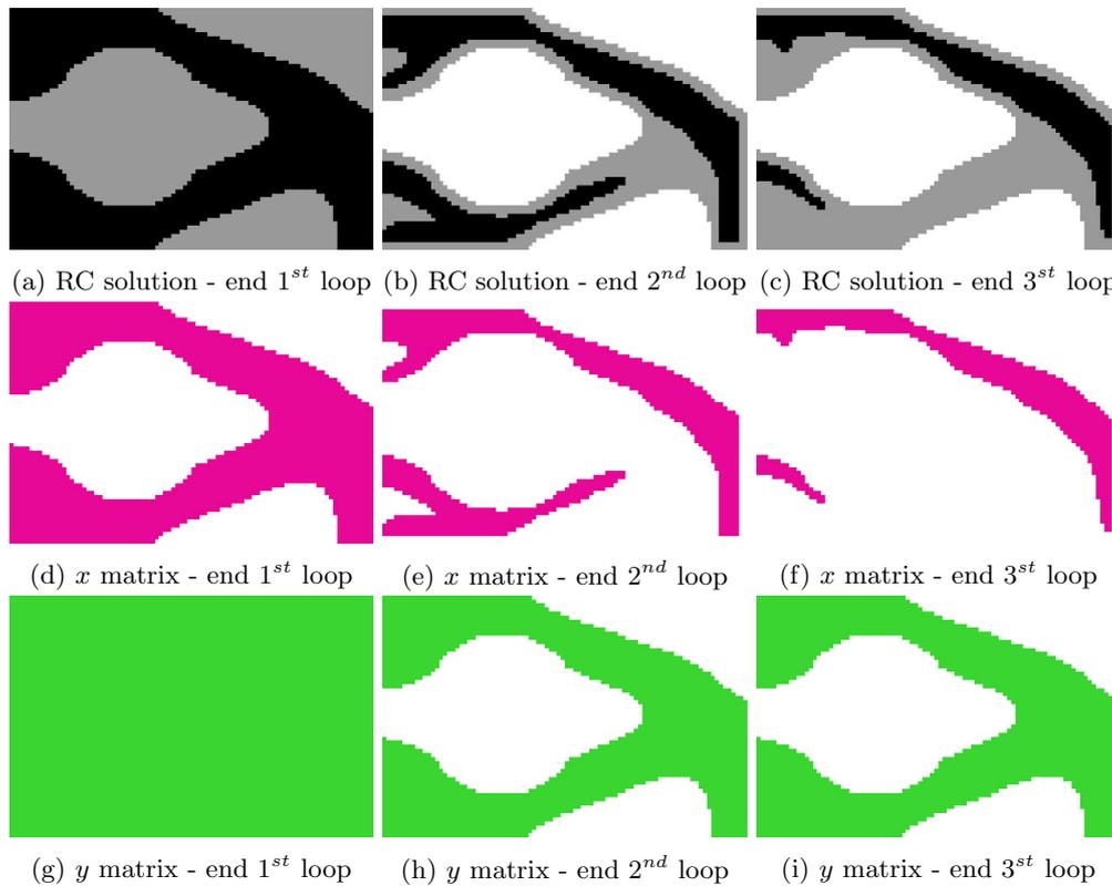
Figure 4.1: Case study n.5 - solutions and matrices  $x$ ,  $y$  for each ESO loop
