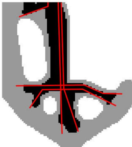
Figure 4.180: Case study n.11 - example interpretation of solution - optimized structure boundaries
