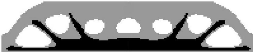
Figure 4.25: Case study n.1 - final solution - optimized structure boundaries
