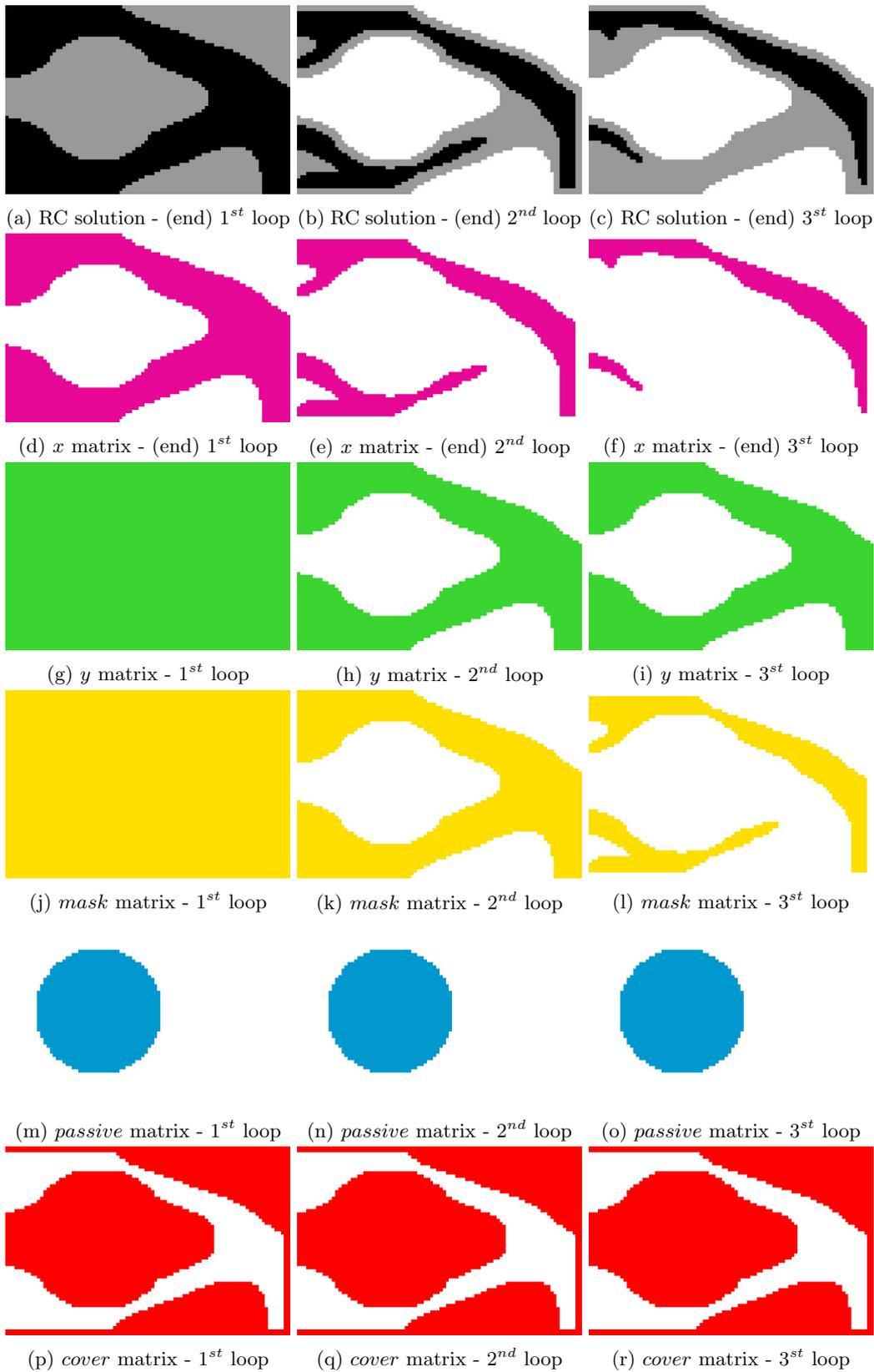
Figure 2.1: Case study n.5 - solutions and matrices  $x$ ,  $y$ ,  $mask$ ,  $passive$ ,  $cover$  for each ESO loop
