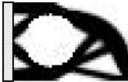
Figure 3.24: Case study n.5 - solution by Sigmund [7] with SIMP stiffness optimization
