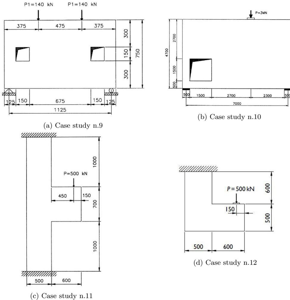
Following in the chapter, there are presented solutions for the above case studies derived by the ESO method of this thesis, along with the solutions taken from literature. All parameters used in the procedure are reported for each case study.
