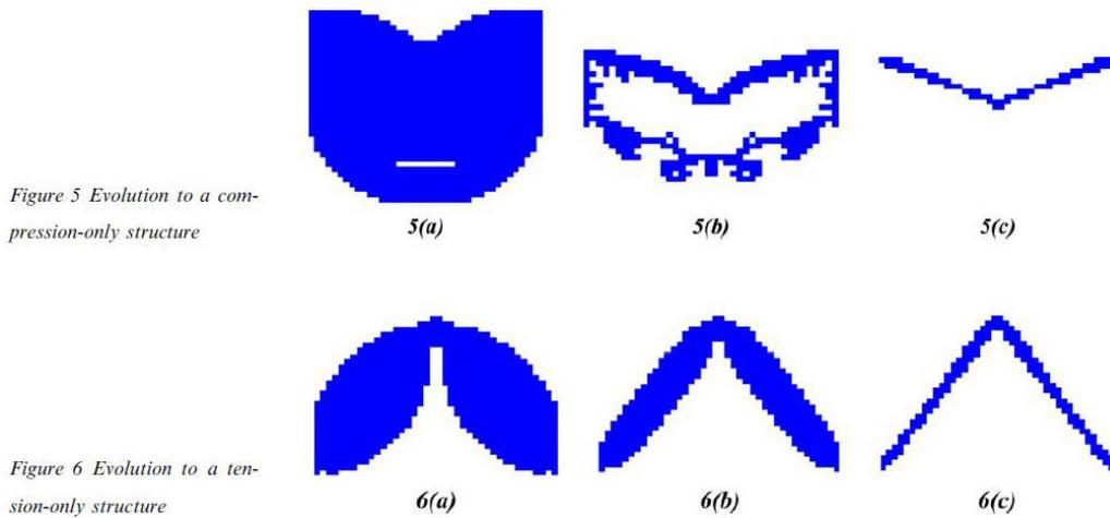
Figure 3.32: Case study n.7 - solution by Xie [17] with first generation ESO optimization with tensile and compressive criteria
