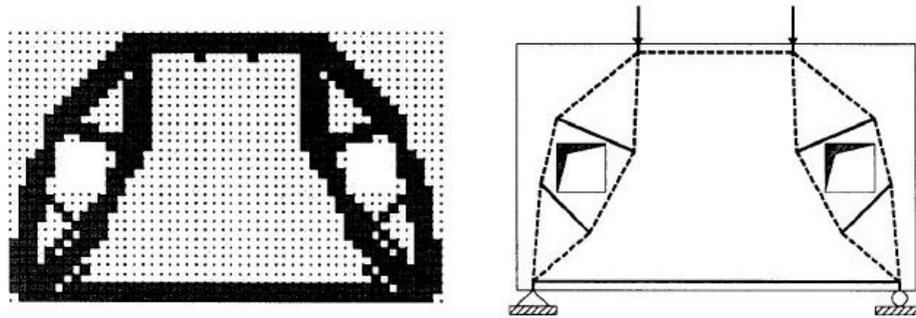
Figure 3.40: Case study n.9 - solution by Xie and Liang [20] with performance based ESO with displacement constraint and resulting strut and tie model
