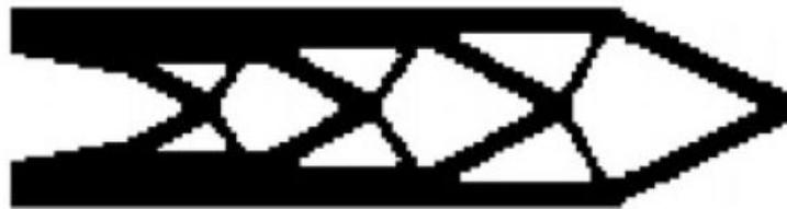
Figure 3.28: Case study n.6 - solution by Xie [18] with ESO stiffness optimization
