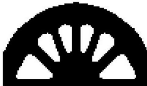
Figure 3.16: Case study n.3 - solution by Xie [11] with ESO stiffness optimization
