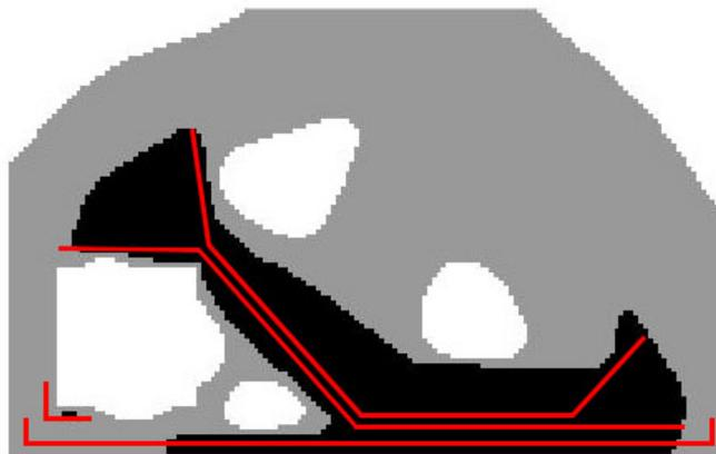
Figure 4.153: Case study n.10 - example interpretation of solution - optimized structure boundaries
