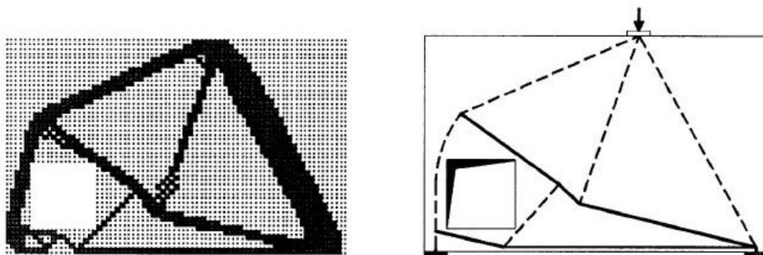
Figure 3.48: Case study n.10 - solution by Xie and Liang [20] with performance based ESO with displacement constraint and resulting strut and tie model
