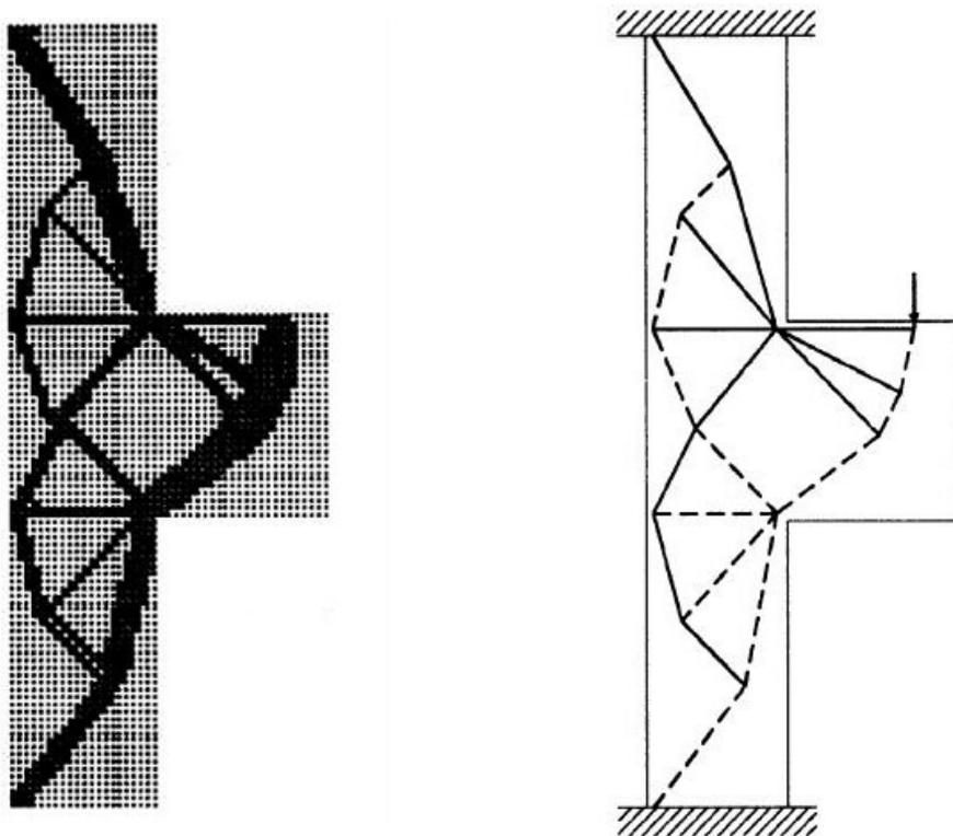
Figure 3.52: Case study n.11 - solution by Xie and Liang [20] with performance based ESO with displacement constraint and resulting strut and tie model
