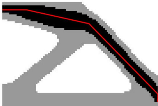
Figure 4.69: Case study n.4 - example interpretation of solution - optimized structure boundaries
