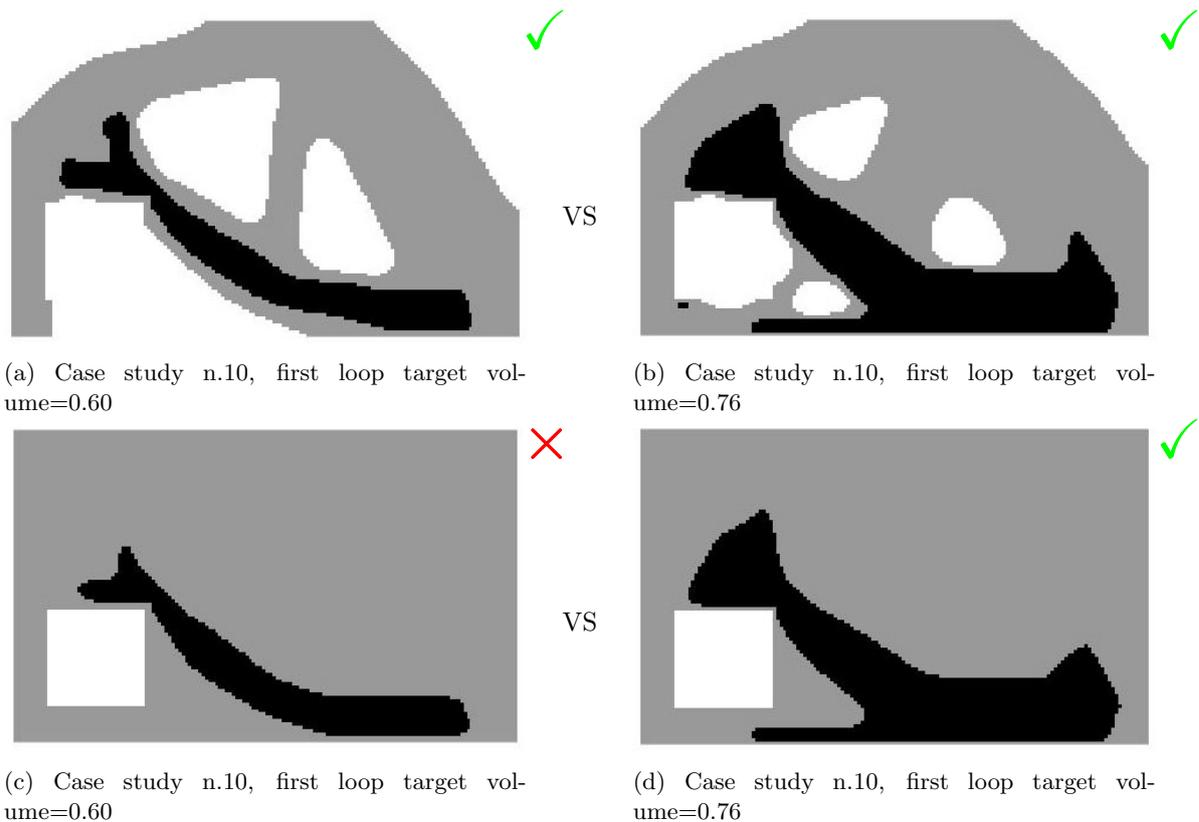
Figure 4.11: Comparison of solutions for case study n.10 with different first loop target volume - with concrete cover
