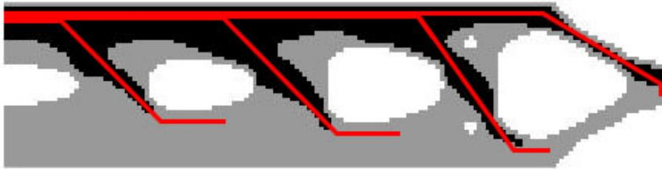
Figure 4.97: Case study n.6 - example interpretation of solution - optimized structure boundaries
