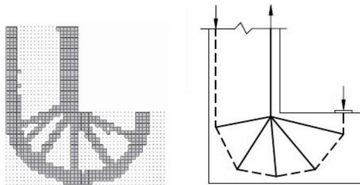
Figure 3.56: Case study n.12 - solution by Liang [4] with performance based ESO with displacement constraint and resulting strut and tie model
