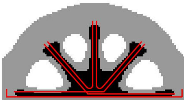
Figure 4.55: Case study n.3 - example interpretation of solution - optimized structure boundaries
