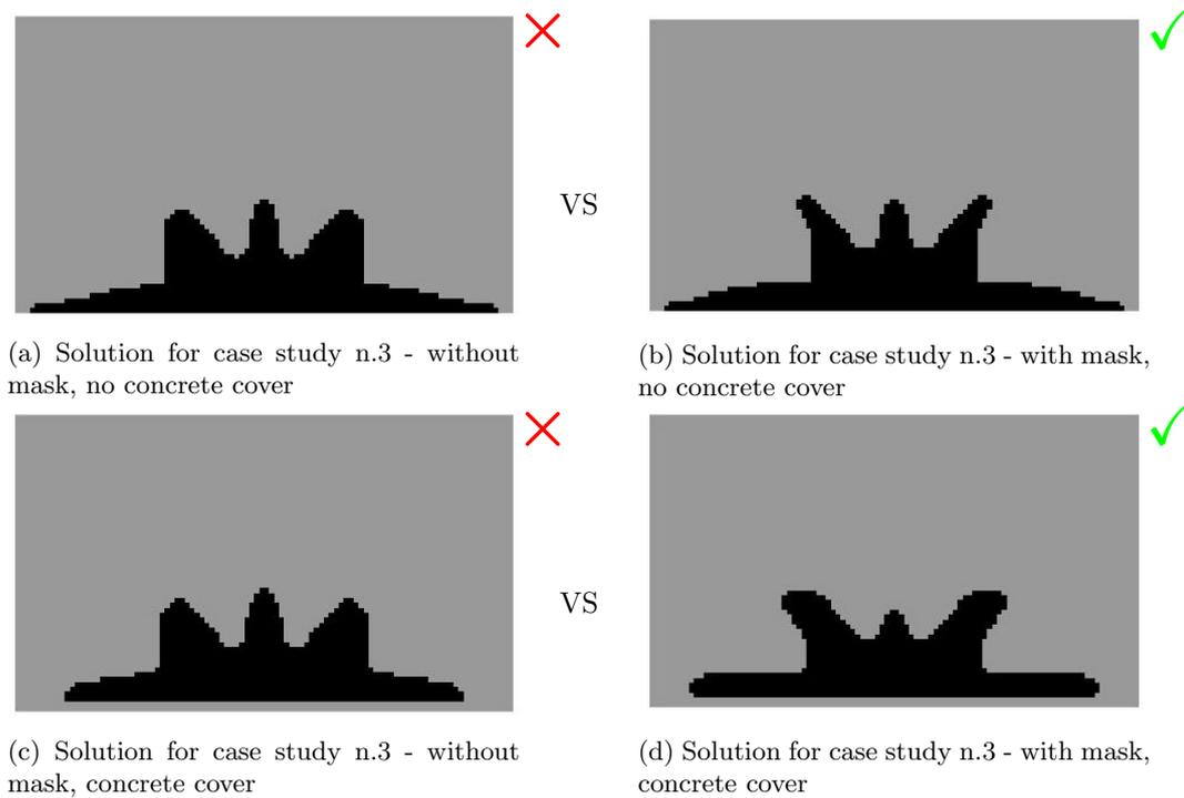
Figure 4.9: Comparison of solutions for case studies with and without mask
