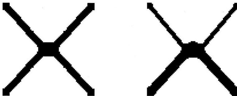
Figure 3.36: Case study n.8 - solution by Xie [19] with ESO stiffness / strain energy optimization with linear and material nonlinear (Drucker-Prager) FEA
