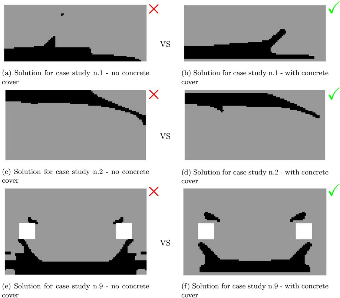
Figure 4.8: Comparison of solutions for case studies with and without concrete cover
