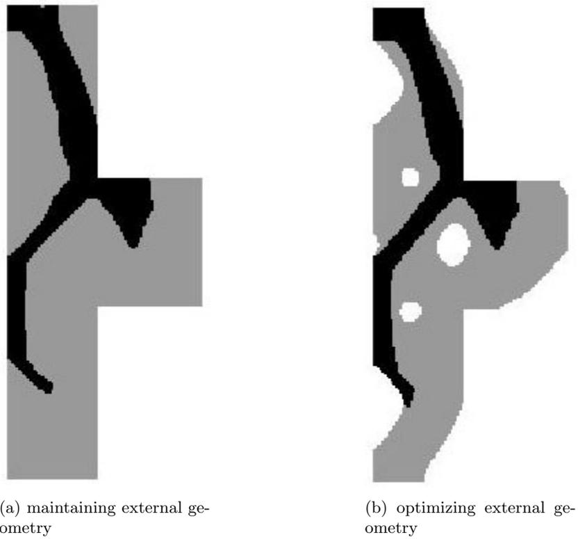
Figure 3.53: Case study n.11 - solution derived by the code developed in this thesis for reinforced concrete - no concrete cover
