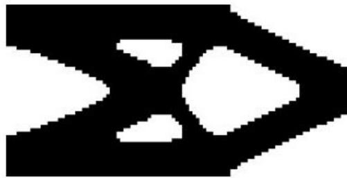
Figure 3.12: Case study n.2 - solution by Xie [11] with ESO stiffness optimization
