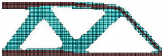
Figure 3.8: Case study n.1 - solution by Xie [10] with multi-material ESO stiffness optimization with materials equally resistant in compression and tension but with different stiffness
