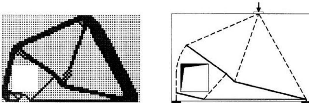
Figure 3.44: Case study n.10 - solution by Xie and Liang [20] with performance based ESO with displacement constraint and resulting strut and tie model
