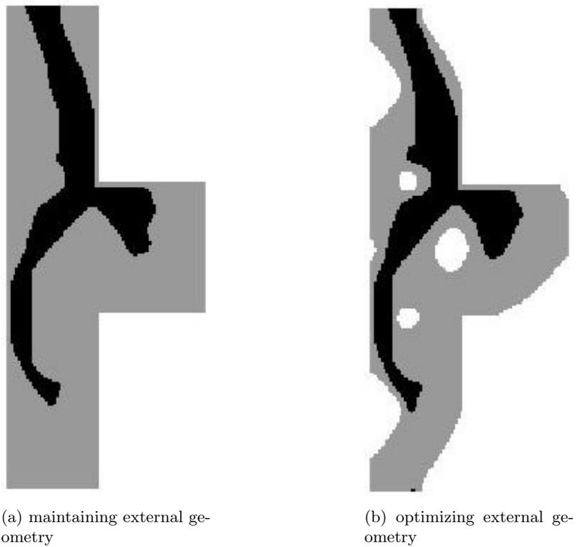
Figure 3.54: Case study n.11 - solution derived by the code developed in this thesis for reinforced concrete - with concrete cover
