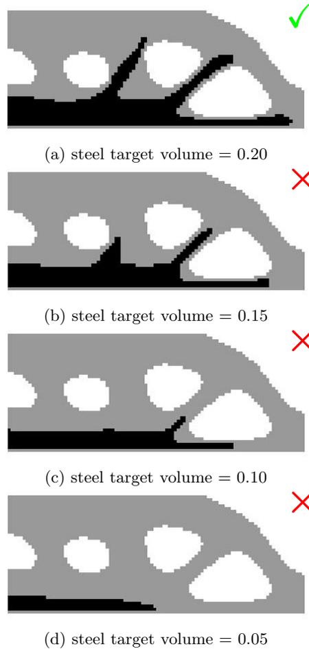
Figure 4.6: Solutions for case study n.1 with different steel target volumes, with concrete cover
