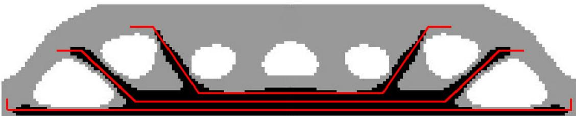
Figure 4.27: Case study n.1 - example interpretation of solution - optimized structure boundaries
