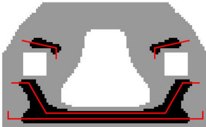
Figure 4.139: Case study n.9 - example interpretation of solution - optimized structure boundaries
