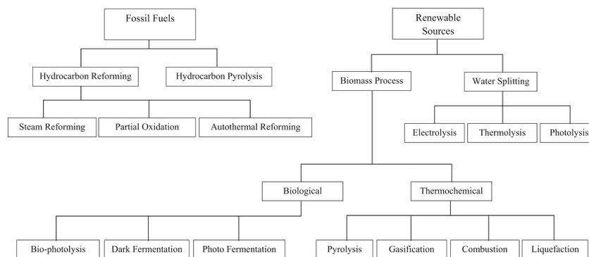
**Figure 3.1:** Hydrogen production processes, (Nikolaidis & Poullikkas, 2017)
