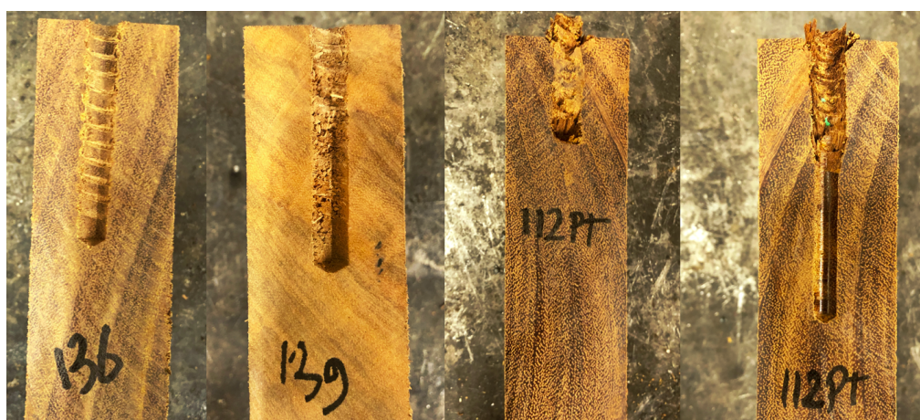
Figure 7.3: (a-first image) Test 136 Kanda with screw diameter 11 mm, insertion depth 70 mm and pre-drilled hole 0,8d. (b-second image) Test 139 Tali with screw diameter 11 mm, insertion depth 70 mm and pre-drilled hole 0,8d. (c-third image) Pre-test 112 with screw diameter 11 mm, insertion depth 50 mm and pre-drilled hole 0,7d; the image shows the other side of the cut. (d-fourth image) Also pre-test 112 but now the full pre-drilled hole is visible.
