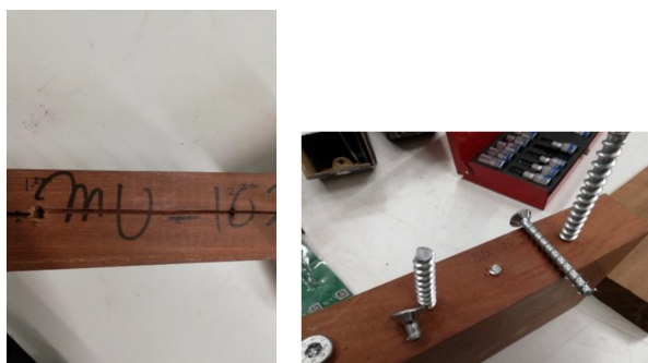
Figure 2.15: (a-left image) Splitting of wood during insertion moment testing. (b-right image) Failure of screw due to insertion moment (Kieboom [15]).
