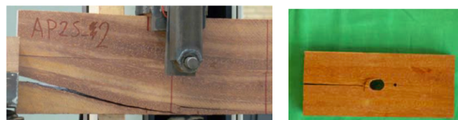
Figure 1.6: (a-left image) Notched beam showing splitting along the grain, with in this case a beam out of tropical hardwood (Ekki) (Kuilen et al. [16]). (b-right image) Dowel connection made out of Ekki showing splitting along the grain after embedment test parallel tot the grain with hss dowels (Sandhaas et al. [26]).
