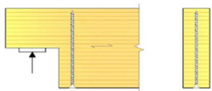
Figure 1.5: Notched beam with self-tapping screws used as reinforcement (Franke, Franke, and Harte [8]).
