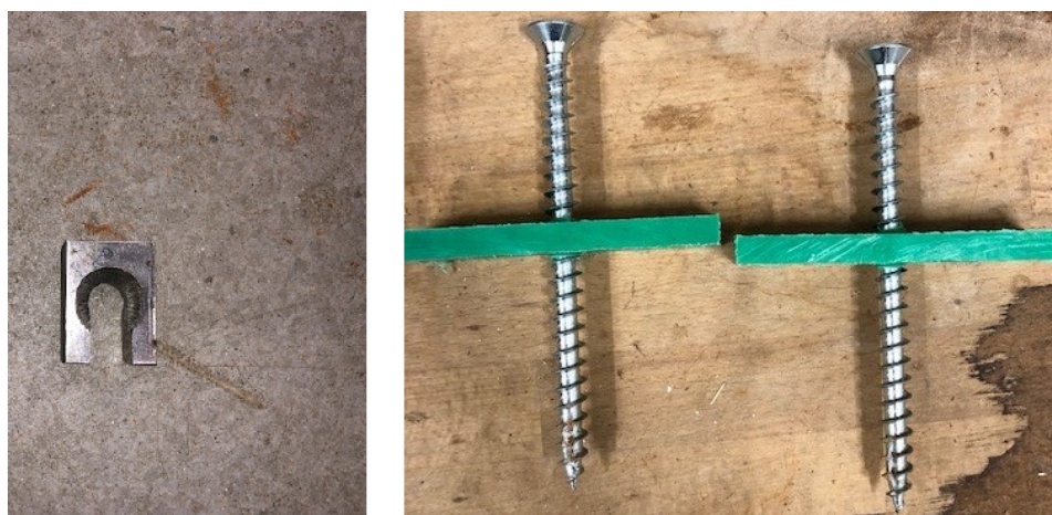
Figure 5.9: (a-left image) Steel piece used to hang the screws in, the tapered hole has the shape of the screw head. (b-right image) Self-tapping screws used in testing; The self-tapping screws are inserted into plastic green parts which are used to support the displacement sensors.
