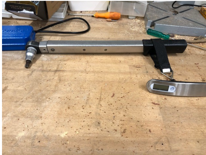
Figure 3.3: Torque wrench shown on the left with the device used to measure the force attached to the handle.
