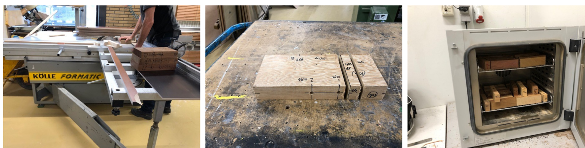
Figure 5.10: (a-left image) Pieces being sawn in the timber workshop. (b-middle image) Original tested specimen cut in pieces. (c-right image) Sawn pieces in dry oven.
