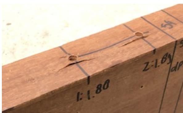
Figure 7.1: Cracks around pre-drilled hole.
