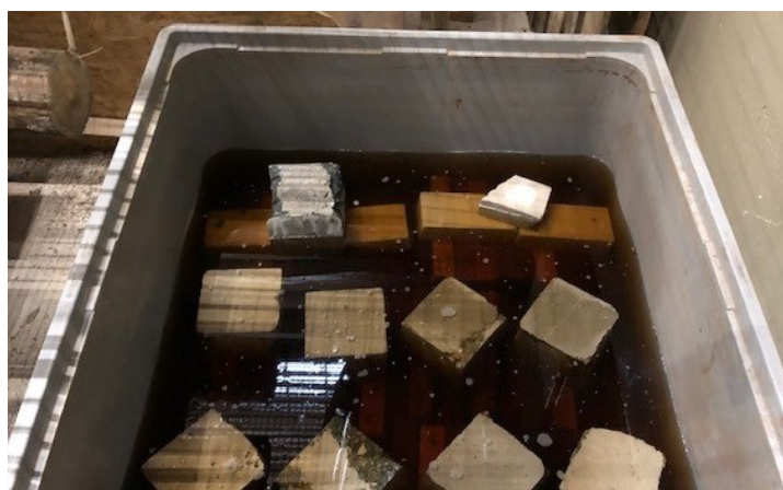
Figure 5.6: Storage of tropical hardwood species underwater, blocks of concrete prevent the pieces from floating.
