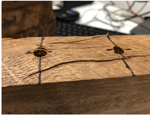
Figure 4.13: Typical failure Limbali.
