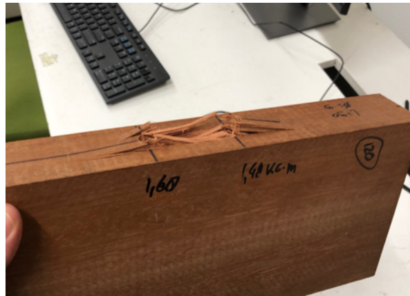
Figure 4.8: Typical failure Mukulungu.
