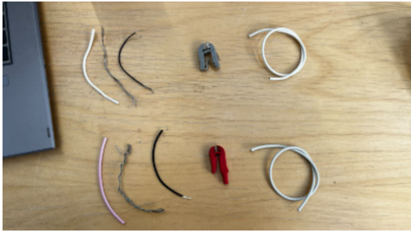
Figure25. Taken apart lead sets for the LCA
