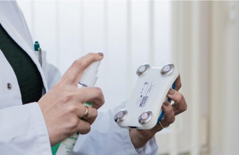
Figure60. Hearteye product using conductive spray
