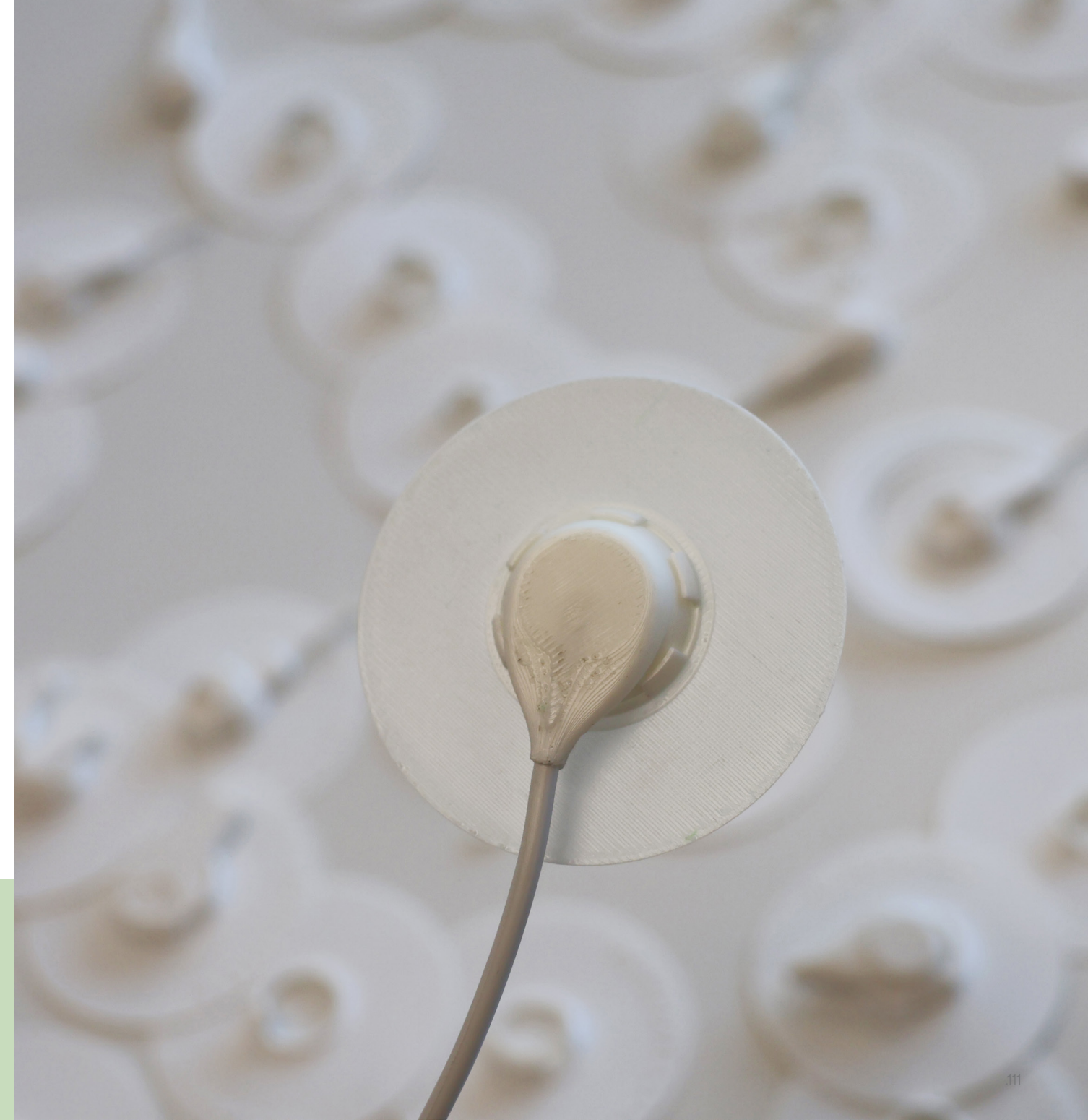
Figure49. Prototype of the electrode and patch
