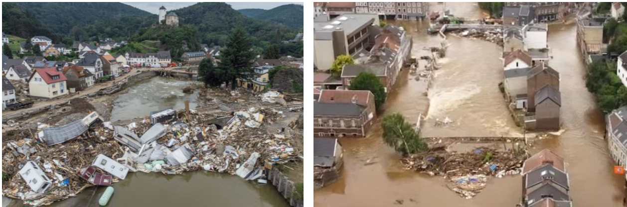
Figure 4: Two extreme examples of debris accumulation, with trees, building rubble, caravans, tanks and other materials show the backwater rise caused by accumulations. Location: Kreuzberg, Germany and Pepinster, Belgium.
