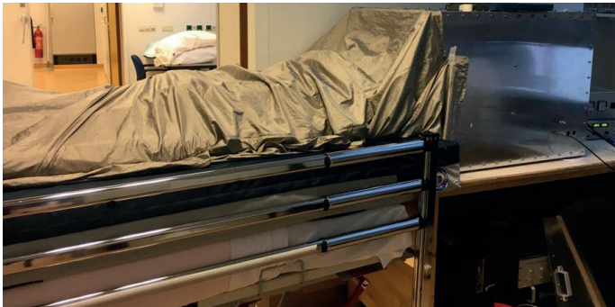
Figure 4.11 Image of person being scanned inside the low field MRI (right) under the conductive shield (left)
