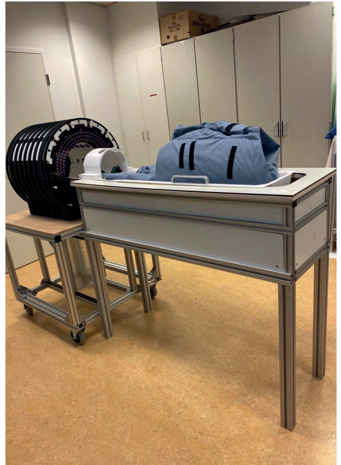
Figure 13.1 Final prototype of bed system with functional magnet system
