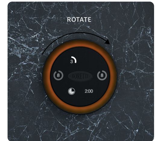
Figure 81: To adjust the time, rotate the ring
