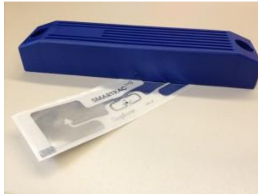
Figure 3-2 Size comparison for a passive and an active RFID tag (source: Atlas RFID Store)
