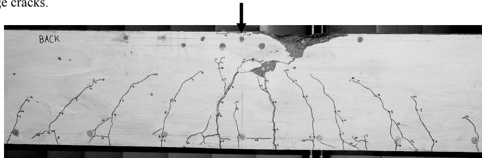
Fig. 6.23: Crack pattern of specimen B45.0.0.N400
