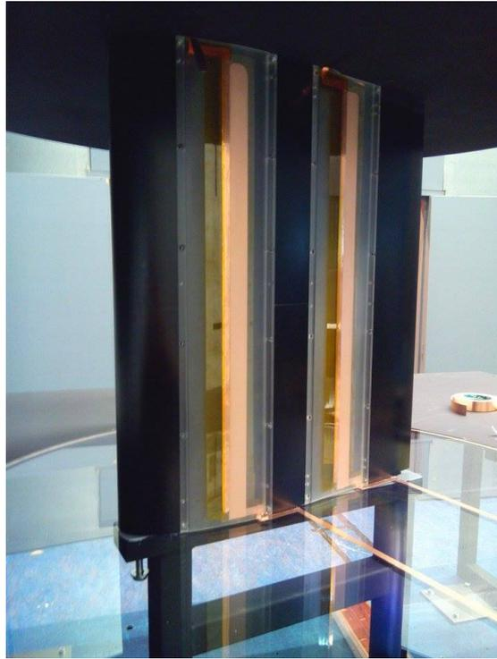
(a) Airfoil model with installed DBD plasma actuators used during experimental campaign.
