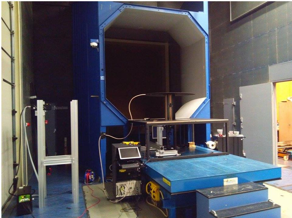
(b) Complete set-up including PIV arrangement, HV amplifier, airfoil model and splitter plate used during experimental campaign.
