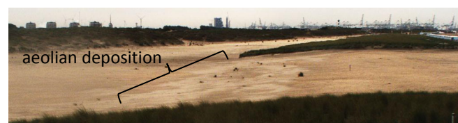
Figure 7. Argus image collected at Vlugtenburg beach (The Netherlands) showing depositional features at the landward side of a dune-like feature created by ground-moving equipment.
