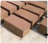
adobe blocks 7% cement 80% laterite 13% water
