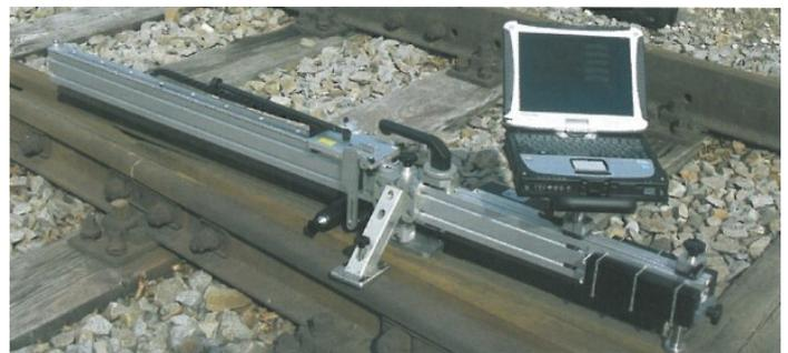
Figure 7 - Wheel dip measurement device [3]
