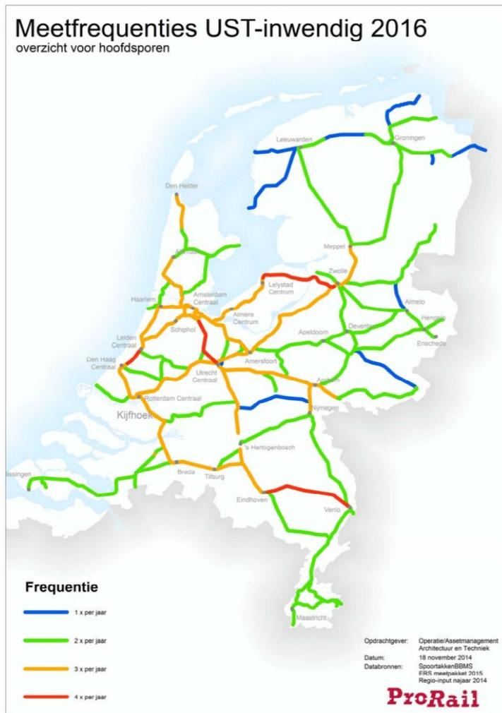
Figure 61 - Frequencies of ultrasonic train inspections [25]
