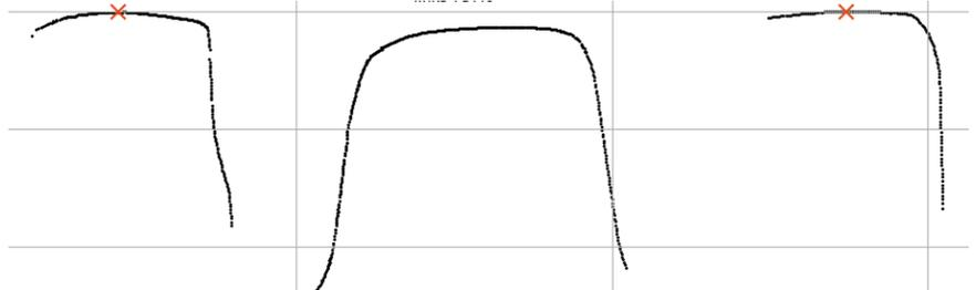
Figure 24 - Rotating based on the highest point on the wing rail
