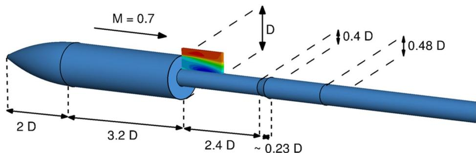
Using the isentropic flow relations, this corresponds to a free stream pressure of 144,186 Pa, a free stream temperature of 260 K, and a free stream velocity ( $U_\infty$ ) of 226 m s<sup>-1</sup>. The Reynolds number based on the model main body diameter ( $Re_D$ ) is 1.3 million. The measurement domain of the simulated experiment has a size of  $1.2 D \times 0.47 D \times 0.08 D$  (60 mm  $\times$  24 mm  $\times$  4 mm,  $L \times H \times W$ ) (see Fig. 3).
