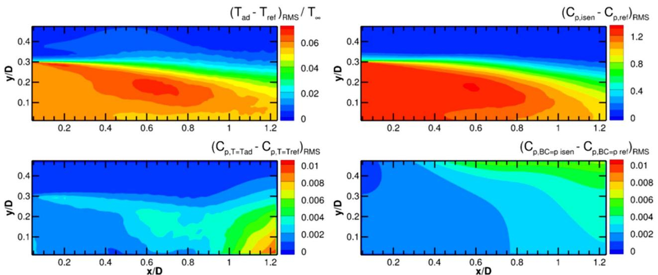
**Fig. 10** R.m.s. difference between adiabatic and reference temperature (top-left); and between pressure from isentropic relations and reference pressure (top-right); impact of using adiabatic temperature
