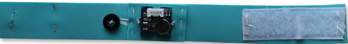
Figure 47: Picture of the user bracelet prototype, currently unconnected to the Seeeduino breadboard
