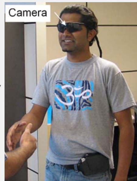
Figure 21: "The prototype Social Interaction Assistant: Hardware"(Krishna, et al., 2008)
