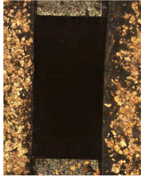
Figure 6.3: Nozzle exit before disassembly under the VK-X1000 microscope
