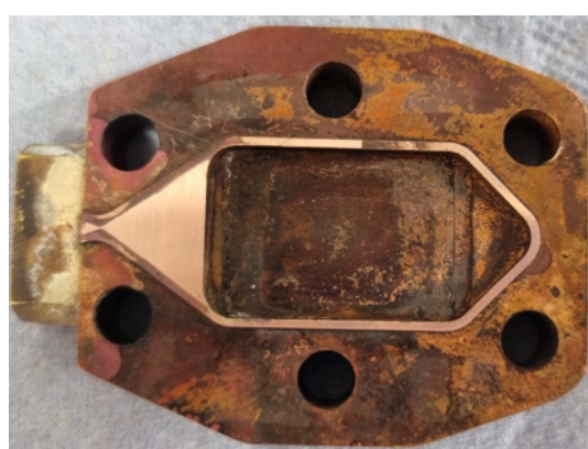
Figure 4.5: Bottom block after polishing with 6\ \mu\text{m}
