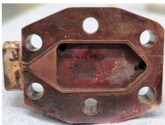
Figure 4.4: Top block after polishing with 6\ \mu\text{m}
