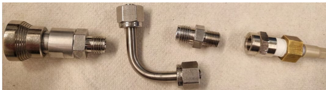
Figure 5.3: Components of the feedsystem inside the vacuum oven
