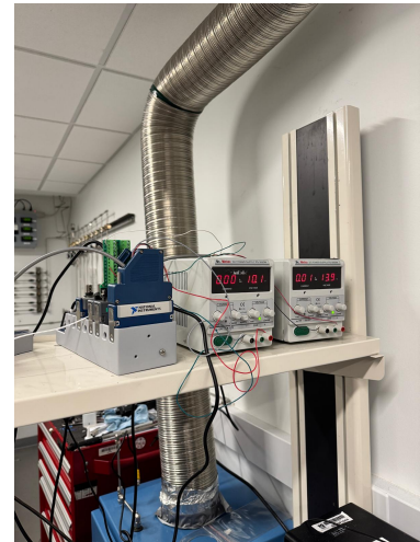
(c) Power supplies and NI modules
