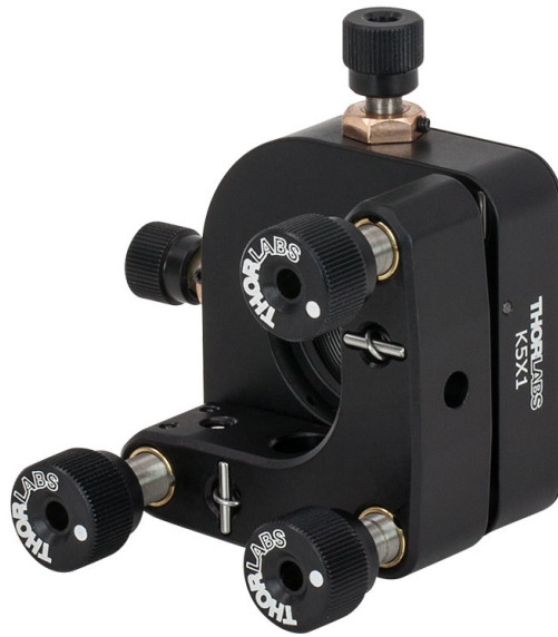
Figure 5.17: Thorlabs K5X1 mount used to hold the SPP. Image taken from [116]
